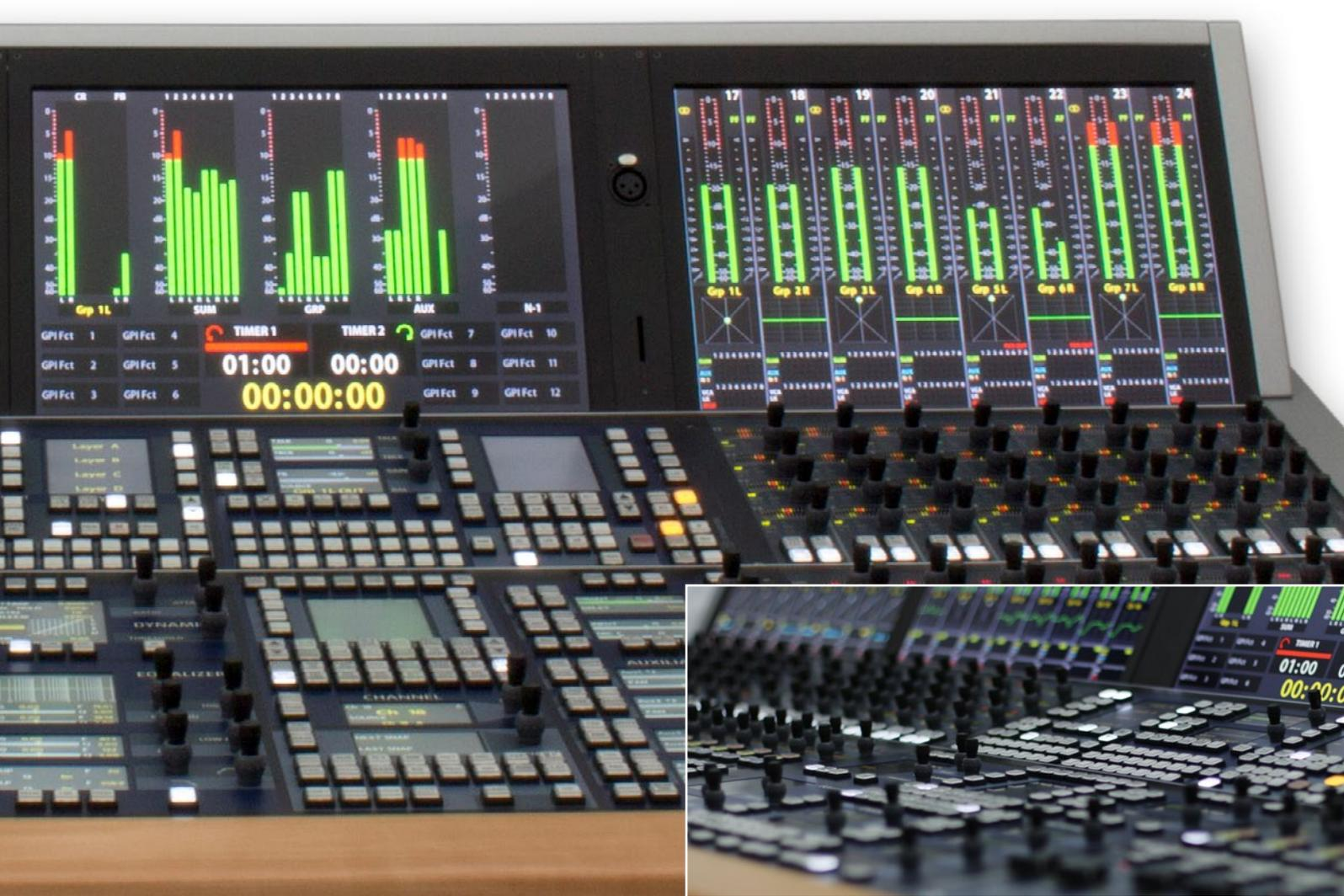
AURATUS is a transportable console and is offered as standard in lightweight construction as a tabletop or built-in version, optionally AURATUS is also available with feet. The mixing console has an extremely low, energy-saving power consumption, even in the largest version with 24 control cables and a central control unit. With 16 control cables, for example, the AURATUS only needs 86 watts. AURATUS therefore does not require a fan. The power supply is always redundant as standard.
